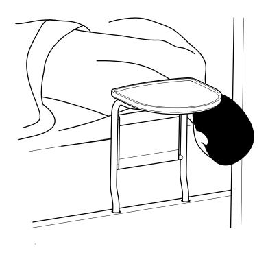
FIG. X1.5 - Zone 5 : Entrapment Between the End of the Rail and the Side Edge of the Head or Foot Board
