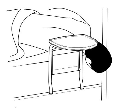
FIG. X1.4 - Zone 4: Entrapment Under the Rail, at the Ends of the Rail
