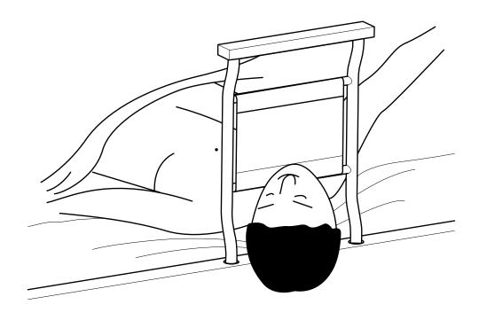
FIG. X1.2 - Zone 2 : Entrapment Under the Rail, Between the Rail Supports or Next to a Single Rail Support
