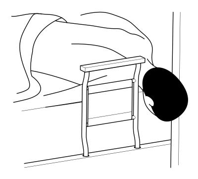
FIG. X1.4 - Zone 4: Entrapment Under the Rail, at the Ends of the Rail
