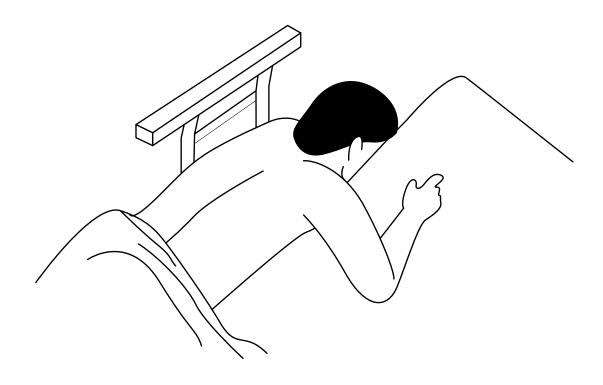
FIG. X1.3 - Zone 3: Entrapment Between the Rail and the Mattress
