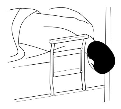
FIG. X1.5 - Zone 5 : Entrapment Between the End of the Rail and the Side Edge of the Head or Foot Board
