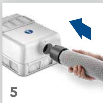
5 Attach the connector to the heating and cooling source by aligning the round opening on the connector to the silver ball on top of the air outlet. Push together until you hear a click.
