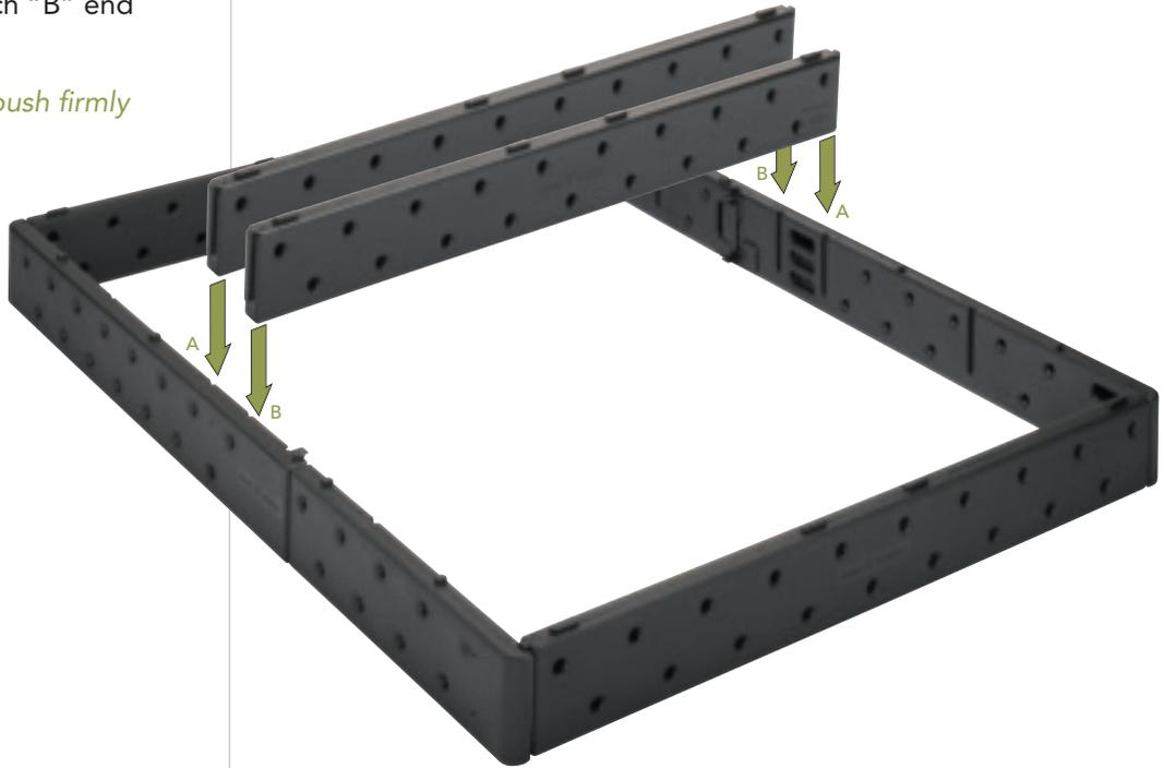
Slide the remaining support beams into the next set of channels.
