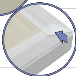
Position the border wrap over foam border walls and air chambers as shown.
