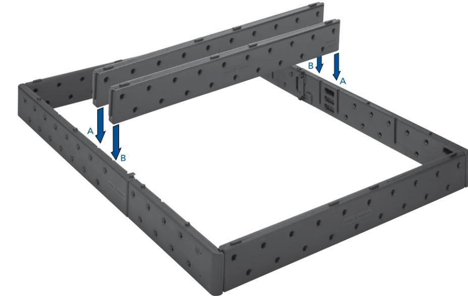
Slide the remaining support beams into the next set of channels.
