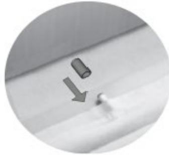
Apply chamber cap to chamber port
