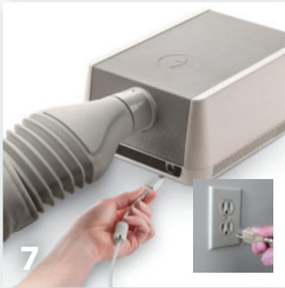
Connect the power cord to the power supply. Plug the power supply into the heating and cooling source with the flat side of the plug facing up. Plug the power cord into a grounded outlet; power light will illuminate and blink for one minute, then turn solid to indicate connection.
